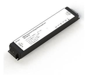
This high-quality 150-watt dimmable transformer for LEDs is ideal for internal applications. Available in a 12-volt model with no minimum load, it is a TRIAC / phase-cut driver, offering LED dimming via a mains 240v power supply and standard household dimmer-switch. (Aurora's AU-DSP400X dimmer module and Varilight's V-Pro series are recommended.)
