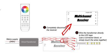
If the LEDs *do not* light up, then the transformer may be faulty. Many of our smaller transformers (internal 30W, 60W and 100W models) have a green light to indicate they are receiving power from the mains supply. If there is no green light, then the transformer is receiving no power or is faulty. Use a voltage
