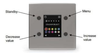
Press top left button to switch between standby / on Press top right "menu" button to select control mode. The display When Sound To Light is active, shows which of the 7 control screens you are currently using: Colour Select - pick one of 10 preset colours
