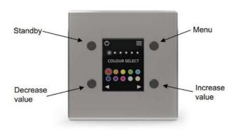
Press top left button to switch between standby / on
