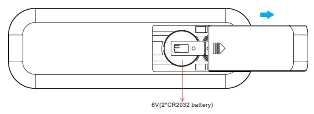
Note:Before the first use, please remove the protective film on the battery.
